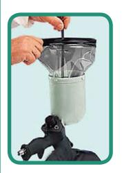
The amount of solvent needed to clean equipment can be greatly reduced by using disposable paint gun liners. Most of the solvent used for spray equipment cleaning is used to remove residual coating from the paint pot. If paint cup liners are used, the residual coating cures in the liner, and is disposed of. This eliminates the need to clean the paint pot. See the "Paint Waste Minimization Fact Sheet" for more information.
